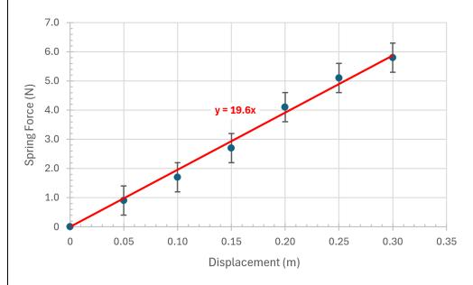
The top of each error bar is the force plus the uncertainty, which is the maximum possible value (assuming we have estimated our uncertainty appropriately). The bottom of each error bar is the force minus the uncertainty, which is the minimum possible value.
