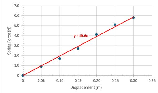
Conveniently, the spreadsheet that was used to plot the best-fit line (trendline) is able to display the equation for the line. The slope is 19.6, which means our spring constant is  $19.6\frac{N}{m}$ .
