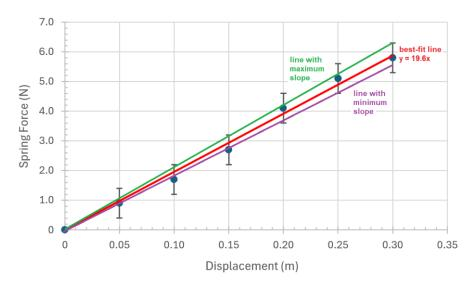
(Note that because zero force must result in zero displacement, the intercept of all of the lines was forced through zero.)
