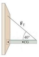
The rope applies a torque to the beam at the end at an angle of rotation with a radius equal to the length of the beam. Gravity applies a force straight down on the beam.
