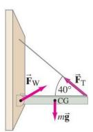
2. Because the beam is not moving (translationally), we know that  $\vec{F}_{net}$  must be zero in both the vertical and horizontal directions. This means that the wall must apply a force  $\vec{F}_W$  to balance the vertical and horizontal components of  $\vec{F}_T$  and  $m\vec{g}$ . Therefore, the vertical component of  $\vec{F}_W$  plus the vertical component of  $\vec{F}_T$  must add up to  $m\vec{g}$ , and the horizontal components of  $\vec{F}_T$  and  $\vec{F}_W$  must cancel.
