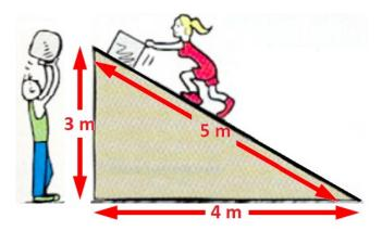
The work that either person does *against gravity* is the change in gravitational potential energy.  $W = \Delta U = mg\Delta h = (2)(10)(3) = 60 \text{ J}$ .
