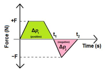
In the above graph, the impulse from time zero to  $t_1$  would be  $\Delta p_1$ . The impulse from  $t_1$  to  $t_2$  would be  $\Delta p_2$ , and the total impulse would be  $\Delta p_1 + \Delta p_2$  (keeping in mind that  $\Delta p_2$  is negative).
