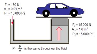
This seems like we're getting something for nothing—we're lifting a car by applying only 150 N of force (approximately 35 lbs.). However, conservation of energy tells us that the work done by  $F_1$  must equal the work done by  $F_2$ , which means  $F_1$  must act over a considerably larger distance than  $F_2$ . In order to lift the car on the right 10 cm (about 4 in.), you would have to press the plunger on the left 10 m.
