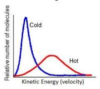
Note that the particles of a substance have a range of kinetic energies, and the temperature is the average. Notice that when a substance is heated, the particles acquire a wider range of kinetic energies, with a higher average.
