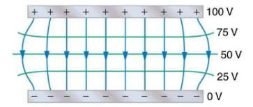
This is the procedure for mapping an electric field. Because electric potential can be measured using a voltmeter, you can use the voltmeter to determine where the isolines are and then draw the field lines so they are perpendicular to the isolines.
