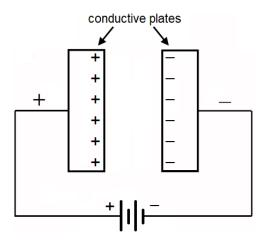
The electrical symbol for a capacitor is a representation of the parallel plates.
