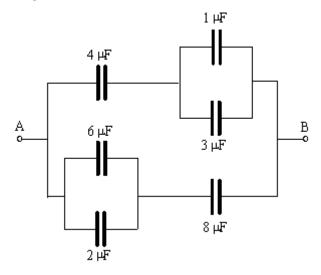
First, we would add the capacitances in parallel. On top,  $3\,\mu\text{F}+1\,\mu\text{F}=4\,\mu\text{F}$ . On the bottom,  $6\,\mu\text{F}+2\,\mu\text{F}=8\,\mu\text{F}$ . This gives the following equivalent circuit:
