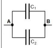
The voltage in a parallel circuit must be constant regardless of the path.
