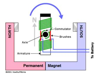
An electromagnet that spins because of its continuously switching attraction and repulsion to the magnetic field produced by a separate set of permanent magnets is called a *motor*. An electric motor turns electric current into rotational motion, which can be used to do work.
