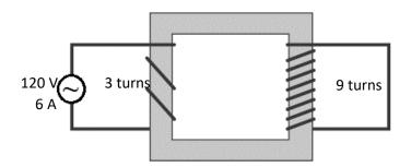
The voltage on either side of a transformer is proportional to the number of turns in the coil on that side. In the above transformer, the primary has 3 turns, and the secondary coil has 9 turns. This means the voltage on the right side will be  $\frac{9}{3}$  = 3 times as much as the voltage on the left, or 360 V. The current will be  $\frac{3}{9} = \frac{1}{3}$  as much, or 2 A.
