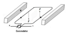
A <u>commutator</u> is used to reverse the direction of the current as the loop turns, so that the combination of attraction and repulsion always applies force in the same direction.
