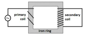
The current on the input side (primary) generates a magnetic field in the iron ring. The magnetic field in the ring generates a current on the output side (secondary).
