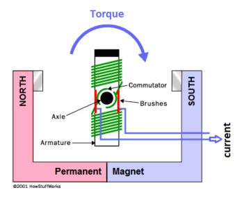
Recall from the previous section that Lenz's Law gives the emf produced by the generator. Because the coil is rotating through a uniform magnetic field, the magnetic flux through the coil is constantly changing, which means calculus is needed to calculate the emf produced.
