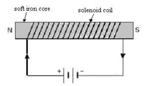
Because the iron core is not a permanent magnet, the electromagnet only works when current is flowing through the circuit. When the current is switched off, the electromagnet stops acting like a magnet and releases whatever ferromagnetic objects might have been attracted to it.
