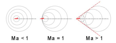
When an airplane is traveling faster than sound, the sound waves coincide at points behind the airplane at a specific angle,  $\alpha$ :
