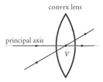
2. Light passing through any part of the lens other than the vertex is refracted through the *focus*.
