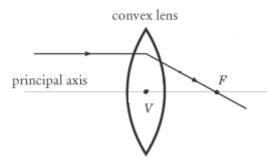
1. If the object is farther away from the lens than the focus, the image is real (on the opposite side of the lens) and inverted (upside-down).
