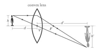
2. If the object is closer than the focus, the image is virtual (on the same side of the lens) and upright (right-side-up).
