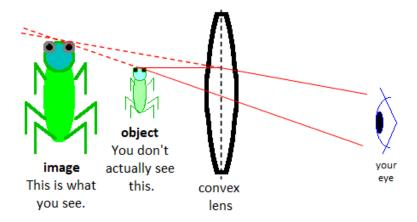
Note also that the lens bends *all* of the light. Your eyes cannot see the unbent light rays, which means you cannot see the actual object in its actual location; you *only* see the image.
