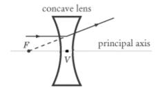
For a concave lens, the image is always virtual (on the same side of the lens) and upright (right-side-up):
