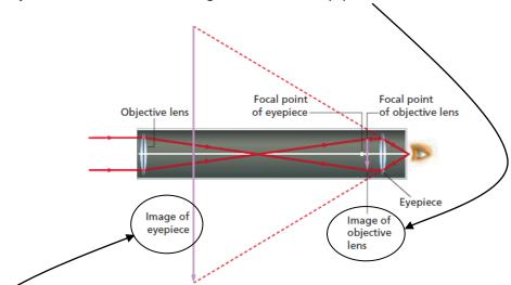
The image from the objective lens is then refracted by the eyepiece. The eyepiece creates a much larger virtual image, which is what the eye sees.
